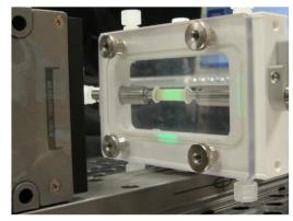
LumeGen Bioreactor Chamber with Laser Micrometer
