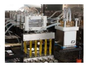
LumeGen Bioreactor System with Six Chambers
